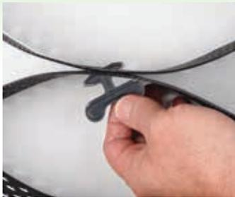
ATRA® keys, made from weather-resistant polyethylene, are 3 times stronger and 3 times faster than stapling. Easy installation: ATRA® keys are inserted through adjoining GEOWEB® cell walls, turned and locked for the most secure connection.
