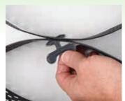
ATRA® keys, made from weather-resistant polyethylene, are 3 times stronger and 3 times faster than stapling. Easy installation: ATRA® keys are inserted through adjoining GEOWEB® cell walls, turned and locked for the most secure connection.
