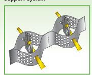
Tendons suspend the GEOWEB® material over geomembranes, hard surfaces, or steep slopes without anchors. Presto uses industry-leading tendons, as tendon type and density are critical to the design strength.
