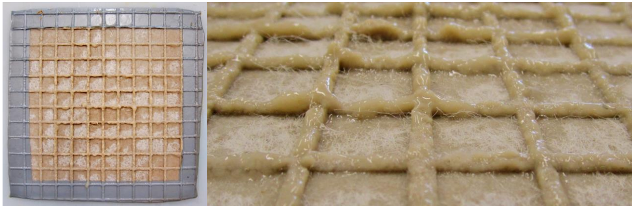
Figure 5. Hydrated bentonite extruded into the grooves of the spacer block after application of 1000kPa
