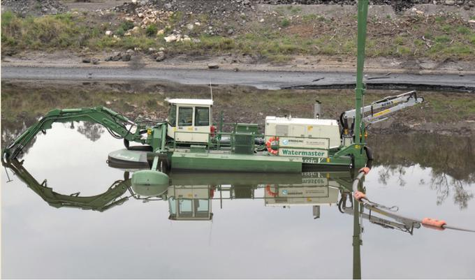
Dredging Systems Pty Ltd was engaged to remove the sludge so that the coal fines could be recovered. A small dredge was used with a rotating cutting head on the inlet pipe. This enables the sludge to slurry in the base of the pond and enables the collection of solids to be accelerated.
