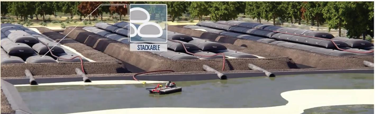
Geotube dewatering containers can be stacked, saving valuable space.
