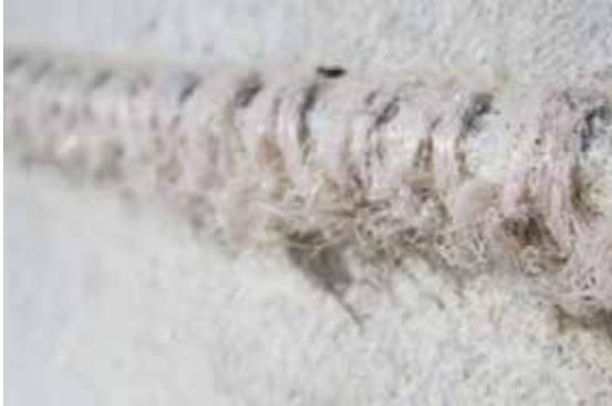
Abraded overlock seam
