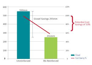
Example of temporary access track showing use of site-won aggregate. Savings of up to 33% include reduction in pavement thickness, as well as lower costs to import fill, casting to spoil and costs to remove large, site-won materials.
