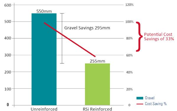
Example of temporary access track showing use of site-won aggregate. Savings of up to 33% include reduction in pavement thickness, as well as lower costs to import fill, casting to spoil and costs to remove large, site-won materials.
